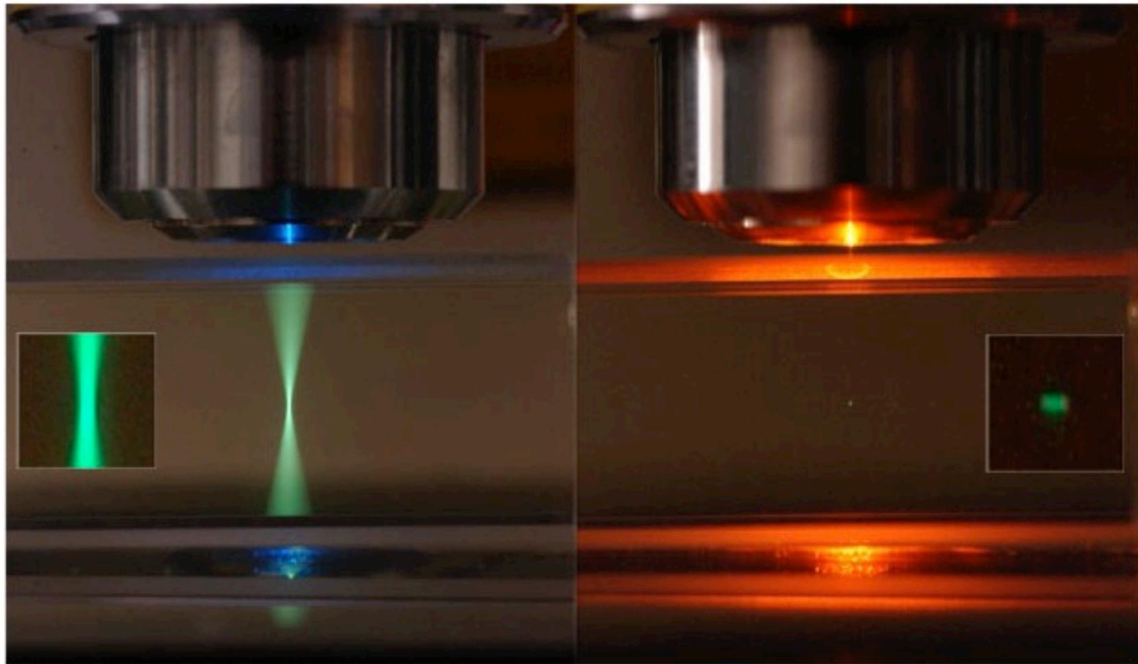
Localized excitation instead of localized emission in a confocal microscope
